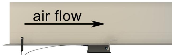
The hole for the air flow sensor is 23mm and should be  $>1$  m in front of the hole for the air hose. The air flow sensor is clamped using the mounting clamp. The supplied foam rubber seal is placed between the duct and the mounting clamp for an airtight seal.
