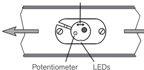
The sensor head must extend into the duct at least 34 mm (max. 115 mm) in the area of the largest air flow speed. Avoid turbulence zones (in front of the sensor  $5 \times D$ , after the sensor  $3 \times D$  distance to disturbing elements).
