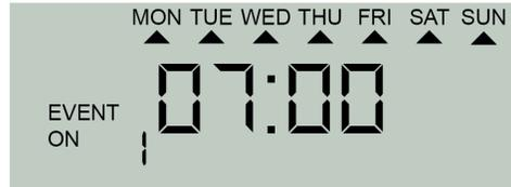
"EVENT ON" means that the device is switched on at this time. "1" means that this is the first of 5 possible memory spaces. The triangles under the abbreviations for the days of the week mean that the device switches on at 07:00 every day.
