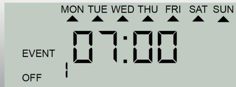
"EVENT OFF" now appears on the display. Proceed as before to set the time. You can no longer change the days of the week here. Press the "MODE" button again to set the interval.
